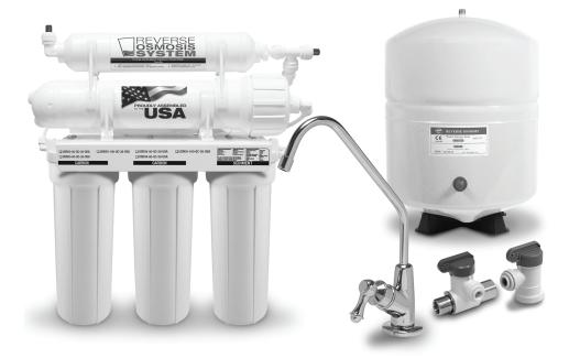
A 5 stage reverse osmosis system for drinking water includes mechanical filtration to remove particles, carbon absorption and adsorption to remove chlorine, taste, odor and chemical contaminants, as well as membrane separation down to .0001 microns. RO membranes remove dissolved solids at the ionic level. No other purification system can provide better removal. Reverse Osmosis Systems provide the best quality drinking water for your family.
