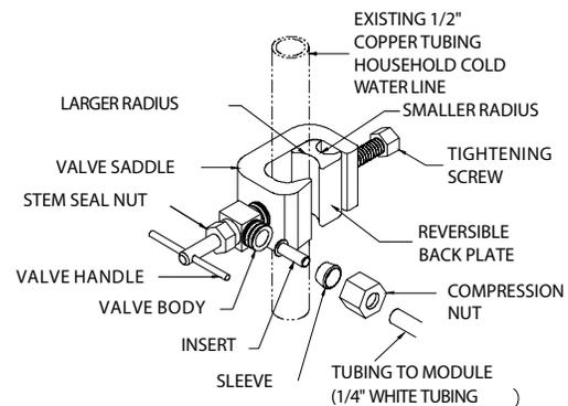
Figure 3: Saddle-Tapping Valve Assembly
