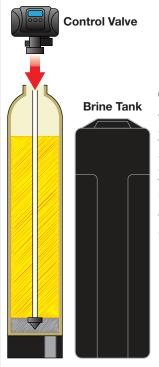
Thread the control valve on to the top of the tank. The control should thread on easily. If you feel any abnormal resistance, check to make sure the control is not cross threaded.
