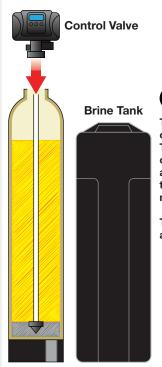
Thread the control valve on to the top of the tank. The control should thread on easily. If you feel any abnormal resistance, check to make sure the control is not cross threaded.
