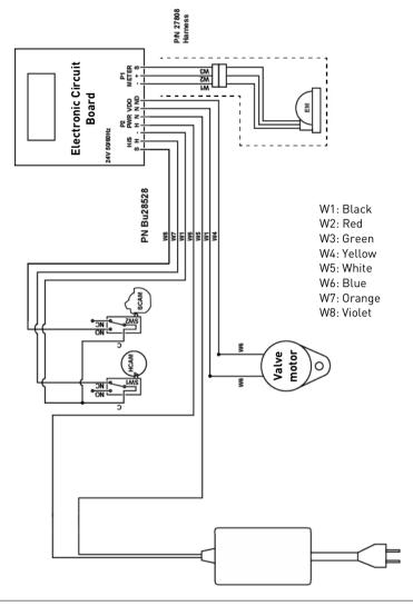
**Note** The microswitch SW2 is connected on C and NO.
