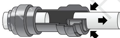
Push in collet against face of fitting and hold. Remove tube. Fitting can be reused
